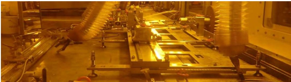
Examination of irradiated fuel takes place inside hot-cells consisting of concrete walls and lead-glass windows over a metre thick. Equipment is operated using remote manipulators and a great deal of skill.
