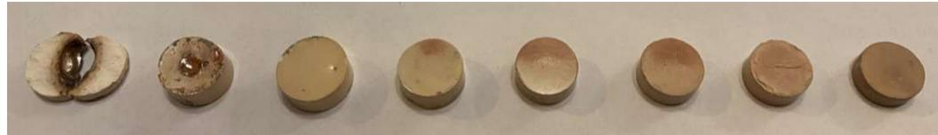
Fig 2. Evolution of CeO<sub>2</sub> pellets under evolving FS parameters. From left to right, localised melting to homogeneous sintering using applied AC electric fields.
