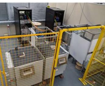
Fig 3. The image of contactless FS furnace including robot and control system
