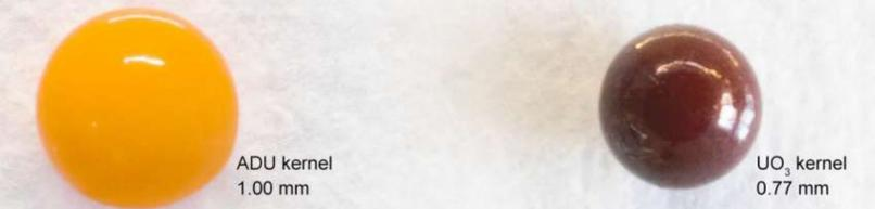
Various casting nib morphologies and sizes have been investigated with the latter having a direct effect on kernel diameter. To date, kernels have been manufactured to a consistent particle diameter of 775  $\mu m$  after calcination.
