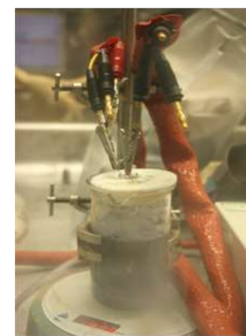
Figure 5: Electrochemical cell: (RHS) diagram of cell (LHS) set up used in glovebox to condition Pu(IV)/Np(V) nitrate.
