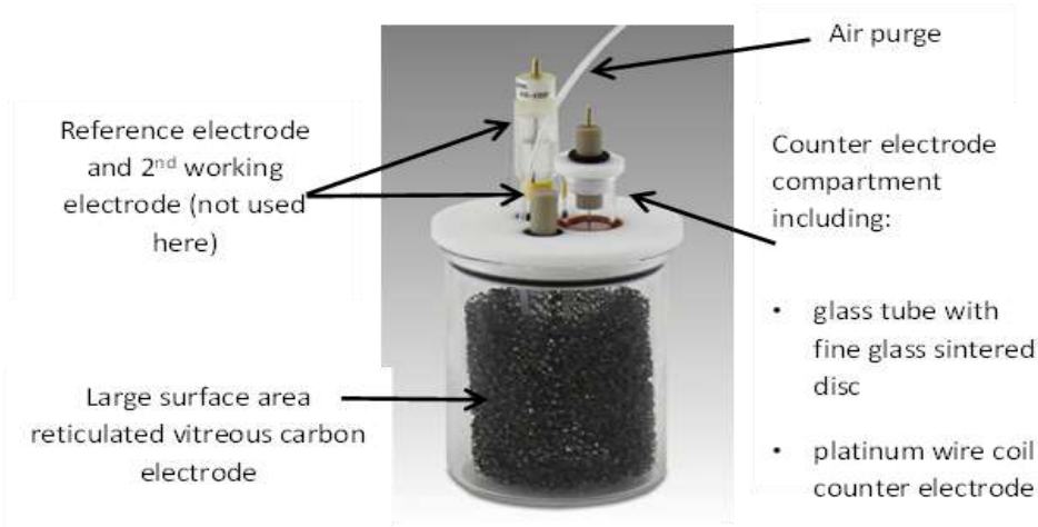
Figure 5: Electrochemical cell: (RHS) diagram of cell (LHS) set up used in glovebox to condition Pu(IV)/Np(V) nitrate.
