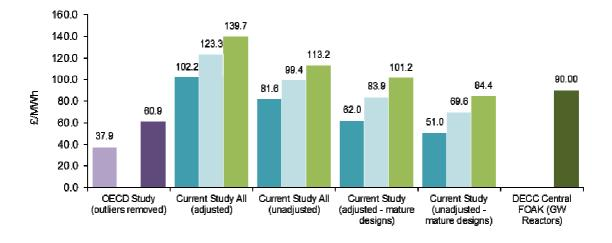
Figure 24 - Levelised Cost of Energy comparison (5%, 8% and 10% discount rates (£/MWh), as at 1 Jan 2012)
