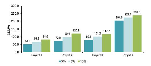
Figure 23 - Levelised Cost of Energy at discount rates of 5%, 8% and 10% (£/MWh, 2012 prices) adjusted, for selected SMRs
