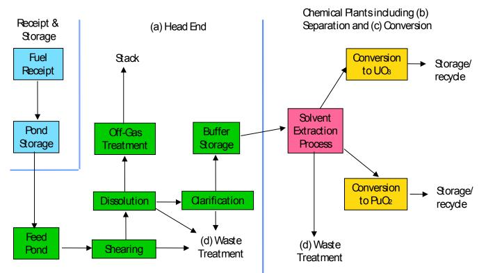
Figure 5: Schematic representation of a typical configuration for an oxide fuel reprocessing plant using the conventional PUREX process, indicating (a) Head End, (b) Chemical Separation, (c) Product Conversion or Finishing and (d) Waste and Effluent Management.
