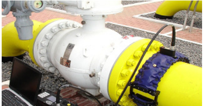
GUL Wavemaker 3 system: inflatable ring with transducers is fitted to the pipe connects to the sampling electronics which are connected to a PC
