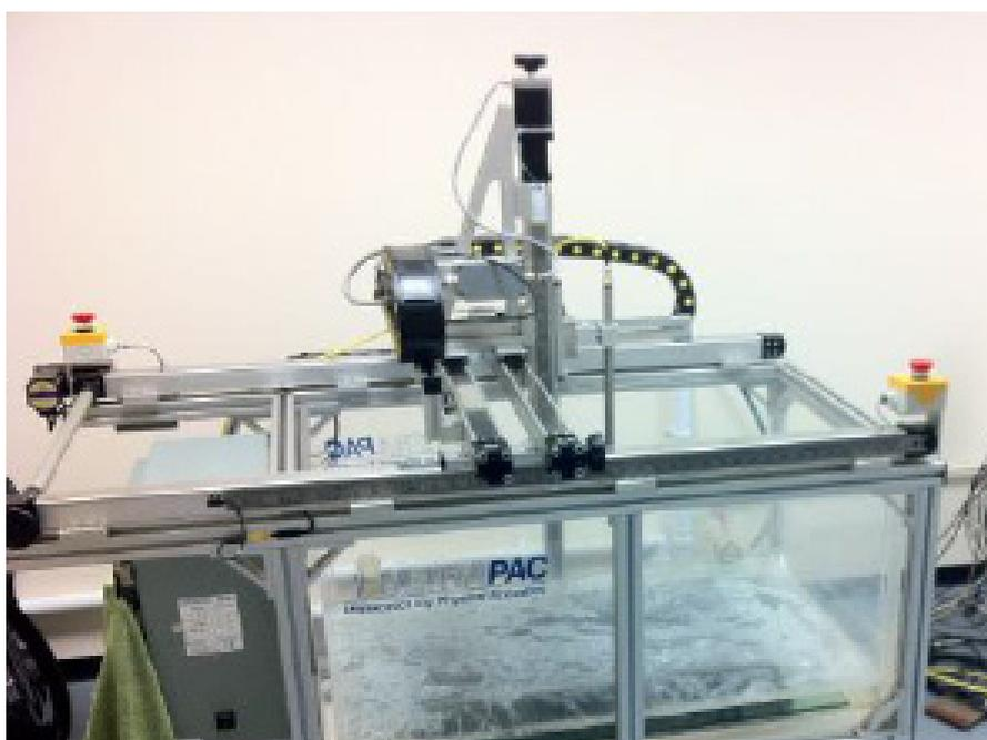
*Immersion tank and scanning frame*
