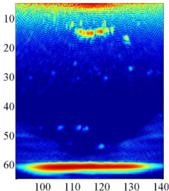
Left: TFM images from Specimen 2 across and along a slag defect
