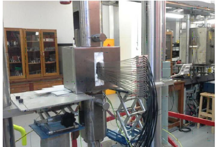
**Above:** Wave guides exiting a furnace containing the sample
